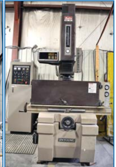
JIN YOUNG EDM Model JDE-45S, SP-50A Control, Work Size 17.7" x 12.6" x 11.8", 3 Axis DRO, Fire Suppression, sn 93031
